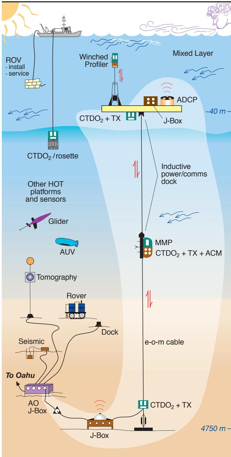
Figure 13. The ALOHA mooring sensor network. The lightly shaded area indicates the 2003 proposed moored sensor network. A similar mooring system has been developed as part of the ALOHA-MARS mooring project.
