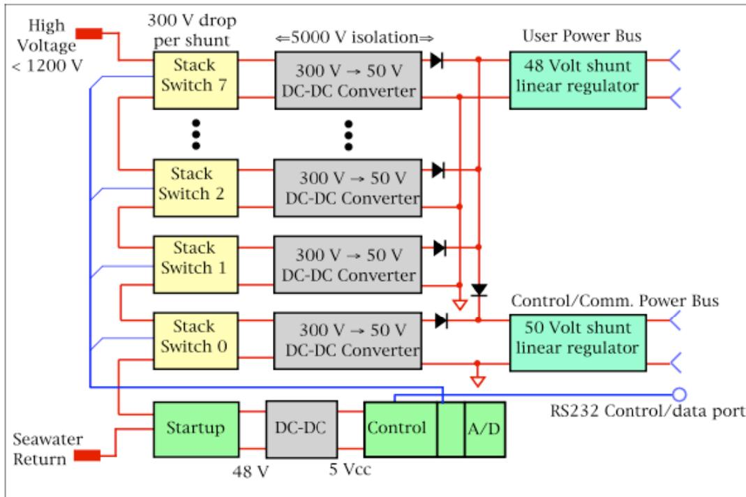
**Figure 3.** The Hawaii-2 Observatory uses a stack of relatively low-voltage (300 Volts) converters to extract sufficient power from the small 370 mA constant current from the cable. At the maximum 1200 Volts, the input power is 444 Watts.
