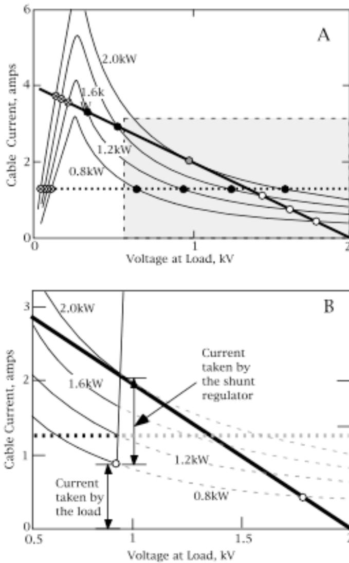
Figure 1. dc-dc Converter operation for a simple hypothetical observatory cable system. Curved lines show power curves for various load demands on a dc-dc converter. A load line for a 2000 V constant-voltage supply is shown as the solid thick line, and a load line for a 1.25 amp constant-current supply is shown as a horizontal dashed line. Stable operating points are shown as small open circles.
