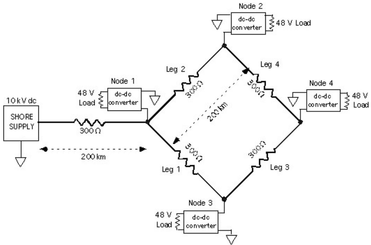
Figure 4. Schematic of PSPICE model for a complex cabled observatory.
