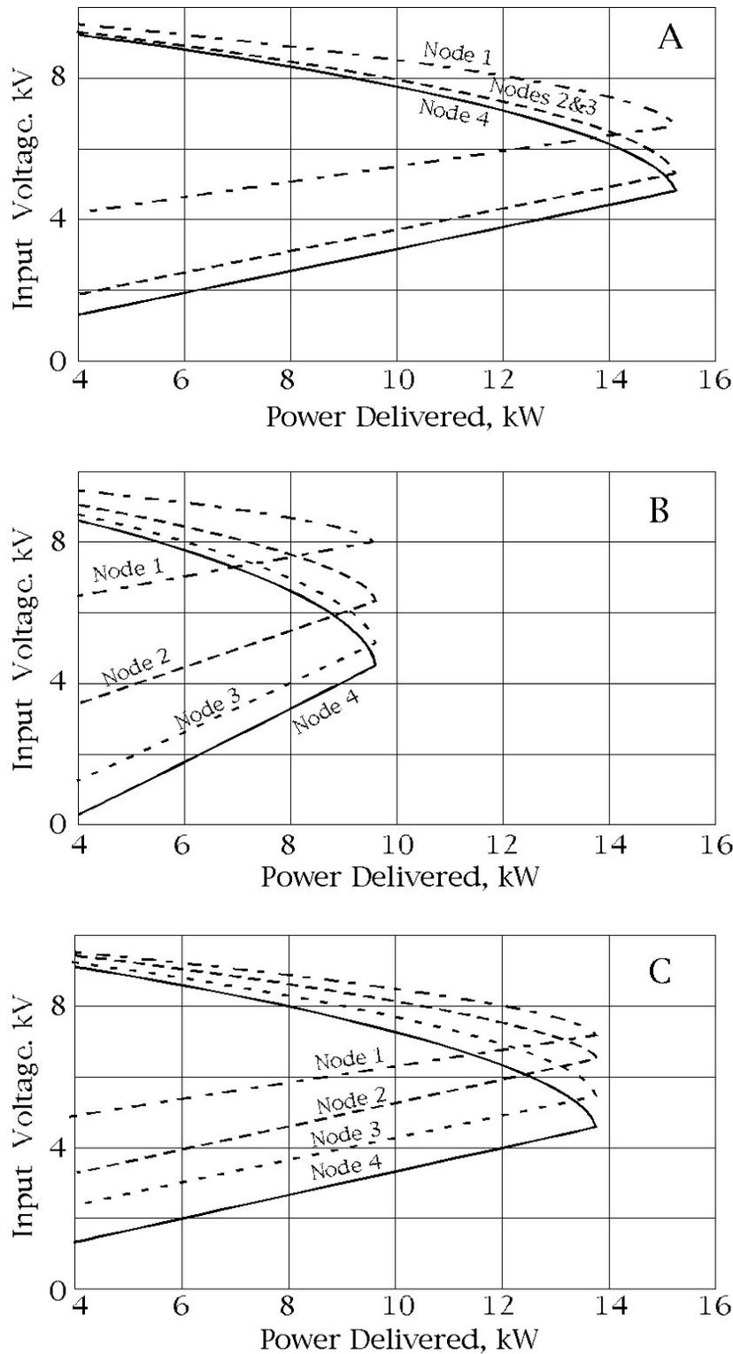
Fig. 5. Model power grid collapse. A): intact array; B): Leg 2 cut; C): Leg 4 cut. The vertical axis is the voltage at the input to each node. In all cases, equal power is delivered to each node, the source voltage is 10 kV, and current is increased until collapse occurs. array now collapses at about 9.5 kW per node (38 kW total). When one of the farther legs (Leg 4) was cut, the remote node no longer has parallel current paths and so the total power is reduced. But since the longest path is
