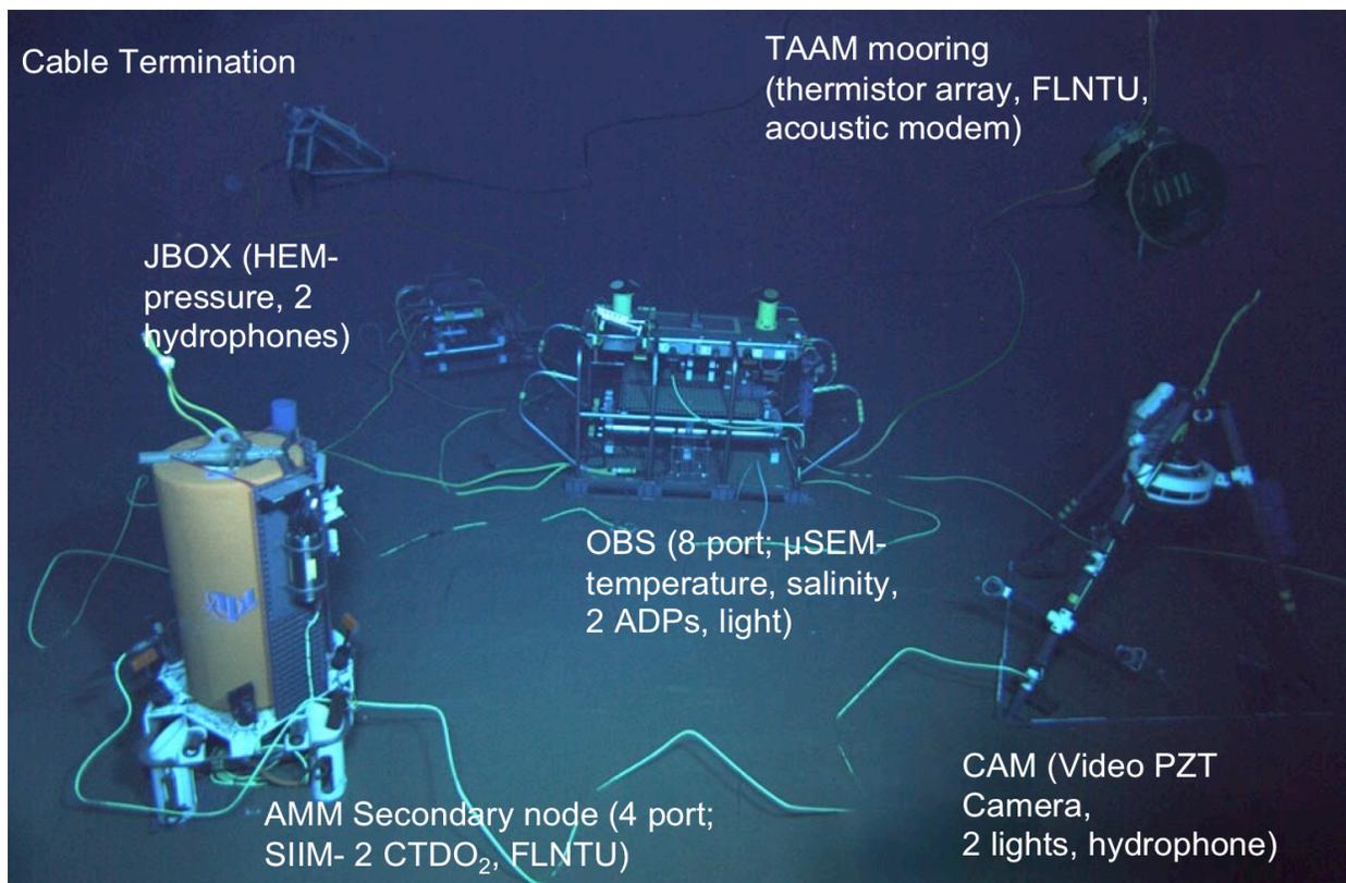
Figure 14. The layout of the ACO system and sensors; the bottom depth is 4728 m (the foreground is true to scale; the cable termination frame and TAAM mooring anchor in the background are farther away, pasted in here). Photo taken by ROV *Jason*.
