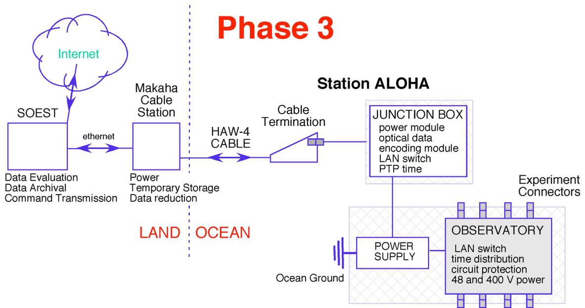
Figure 4. The ACO block diagram for Phase 3.
