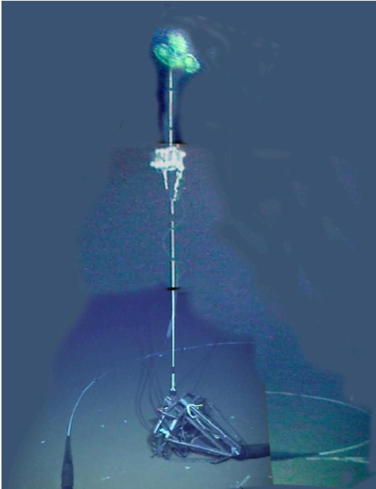
Figure 2. The ACO sea cable termination and proof module. The proof module with hydrophone and pressure sensor and the seawater ground are on the short mooring that was deployed in February 2007. ROV Jason took this composite image in October 2008.
