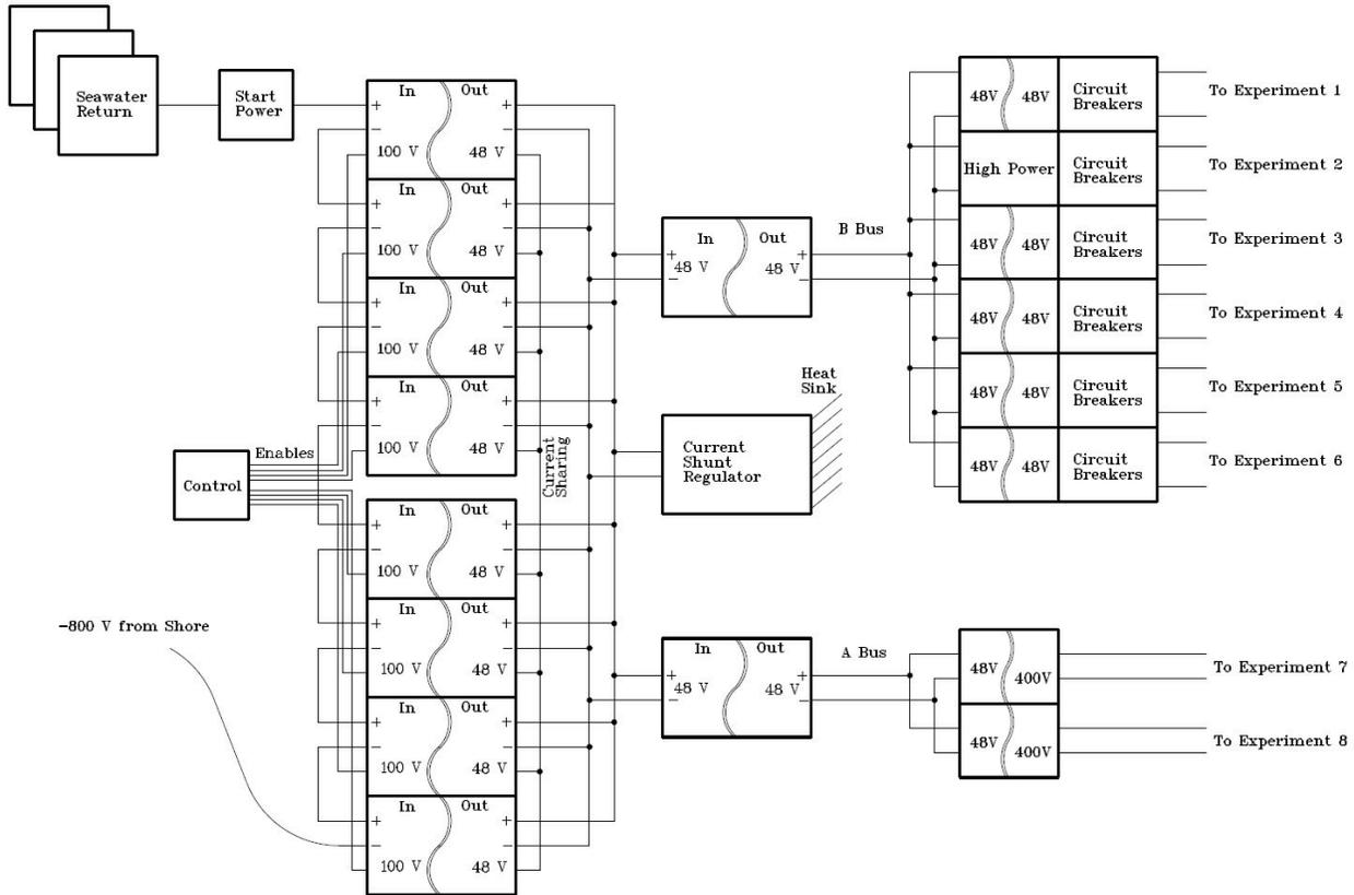
Figure 5. The ACO power supply block diagram. The observatory uses a stack of relatively low-voltage (100 V) converters to extract sufficient power from the 1.6 A constant current flowing through the cable.
