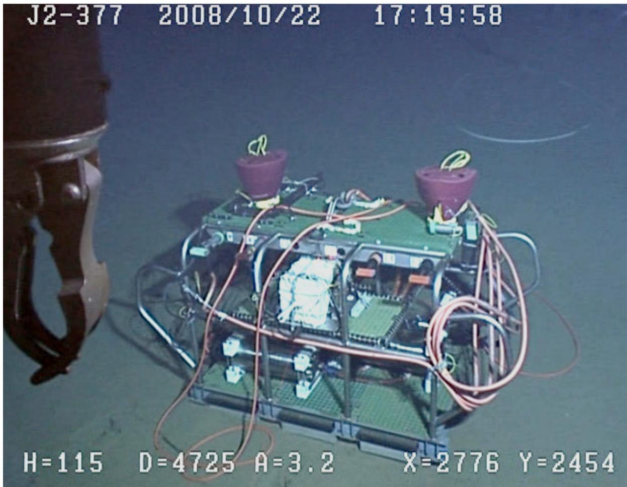
Figure 3. The ACO observatory module. ROV Jason took this photograph in October 2008, just after the module was set on the bottom.
