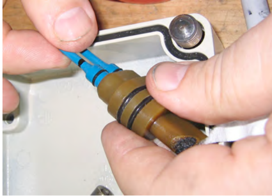
Figure 2. Optical feed-thru in B1 NRH flying connector. Leakage around or through this assembly resulted in an electrical short (blackened area on right).
