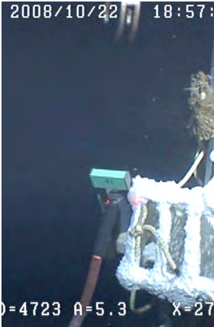
Figure 4. Proof Module Umbilical in the holster on the Proof Module. A stream of oil bubbles can be seen rising from the right side of the connector. [Jason-2 frame grab.]
