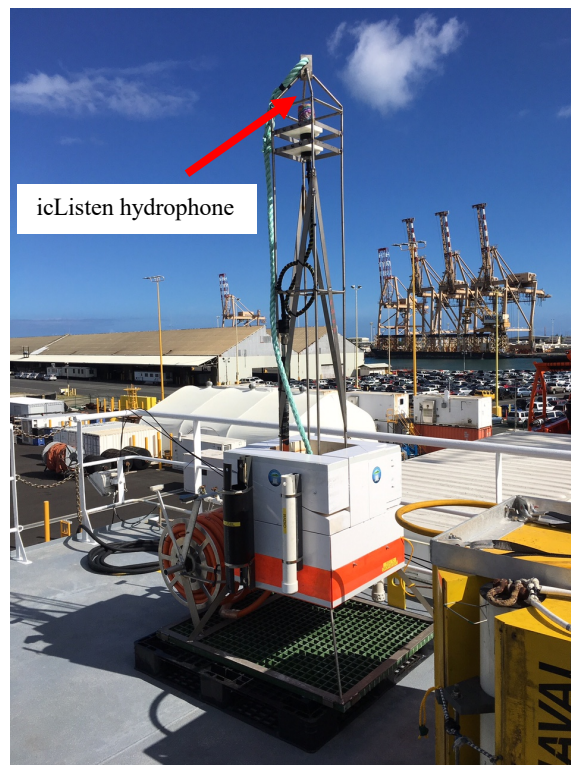
Figure 14. Basic Sensor Package 3 (BSP3) before deployment. The icListen hydrophone is vertically mounted at the top of the metal frame, with a flow-noise reducing “sock” over it. The height from the ground to the mounting is 2.60 m.
