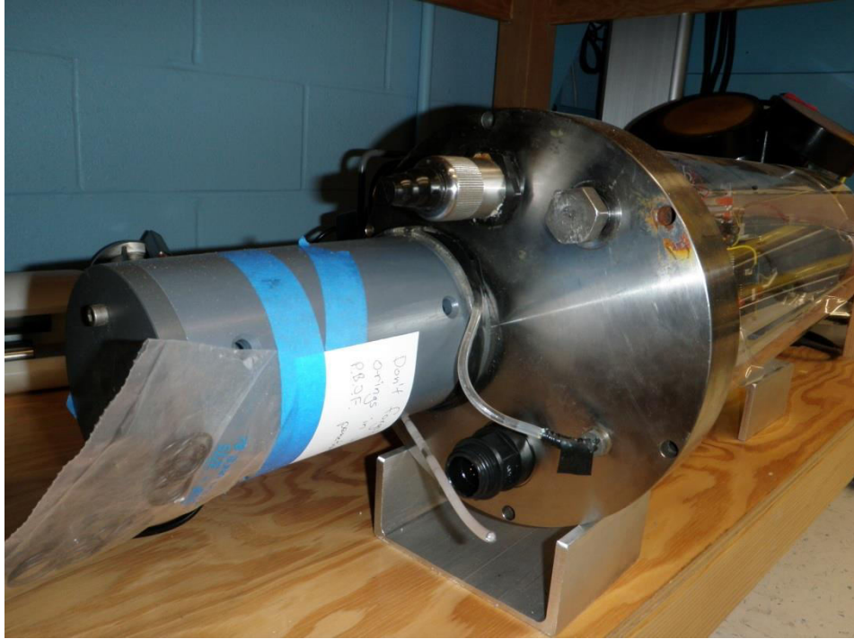
Figure 3. HEM pressure case that the hydrophone is mounted to; it is inside the PVC case.
