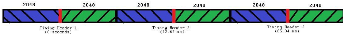
Figure 6. Symbolic representation of the how the hydrophone's 96 kHz data is stored. The blue rectangles correspond to the first 2048 data points collected. The red rectangles represent the headers containing the timing information. The green rectangles correspond to the next 2048 data points collected.
